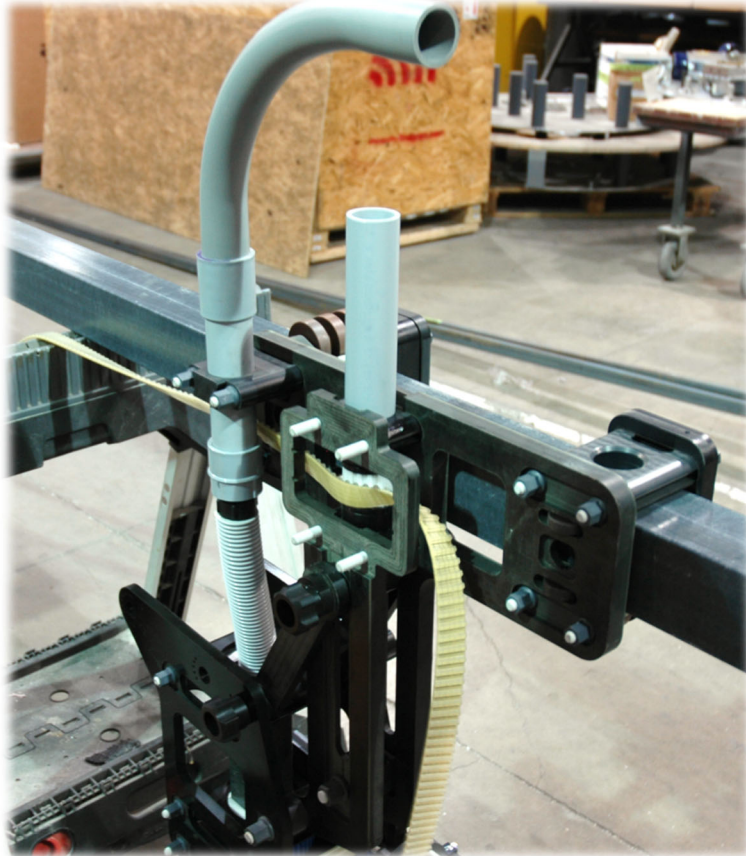
Thread the belt over the timing pulley.
